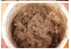
In case of volumetric product, clay core is modelled in the shape of the desired product and the model is wrapped Thoroughly by a layer of wax mixture and detailed with the asphalt mixture (by heating them in chulha). The model is left to dry in the sun. On the other hand, in case of flat product, the model is directly made and detailed out of a layer of two mixtures (by similarly heating them in chulha).
