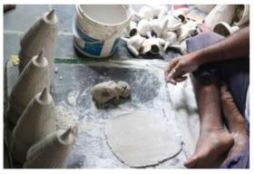
The mixture is laid flat by a roller. Shining powder is sprinkled over it.
