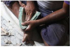
Flat layer is pasted on the cement mold and pressed into the details.
