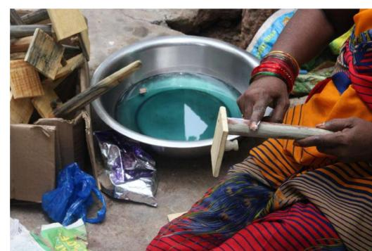
It is dipped in Kerosene to make it pest and termite resistant.
